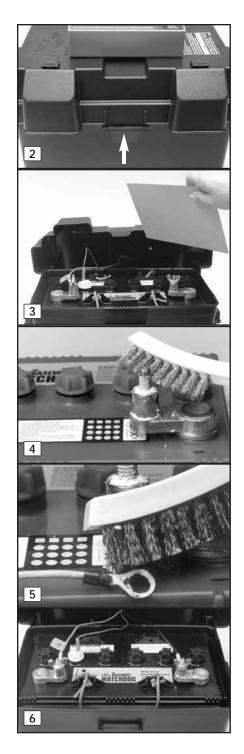
cap, replace it now. Then, replace the battery cables, BLACK to the NEGATIVE (-) post, and then RED to the POSITIVE (-) post. Tighten the wing nuts.
