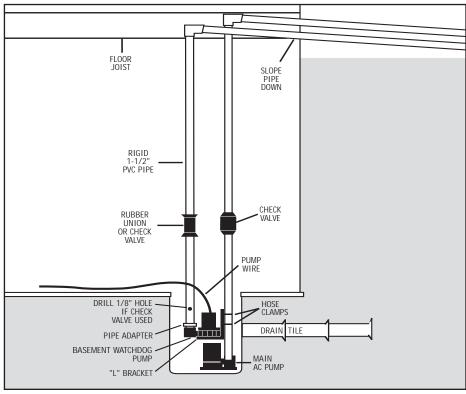
INSTALLATION D: HOOKUP TO EXISTING DISCHARGE PIPE FOR NARROW SUMP PITS (Diagram D)
