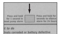
To test the pump, press the YELLOW button for 1 second. The pump will run for 25 seconds and then shut off automatically.
