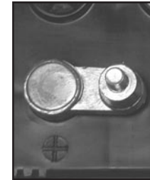
POSITIVE POST HAS LARGER DIAMETER
