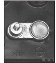
NEGATIVE POST HAS SMALLER DIAMETER
