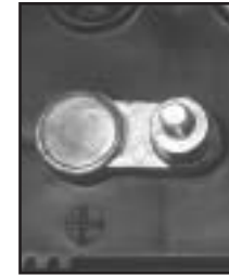
POSITIVE POST HAS LARGER DIAMETER
