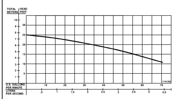
Testing is performed with water specific gravity of 1.0 @ 68°F (20°C), other fluids may vary performance
