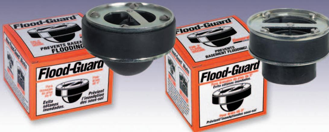
**F**lood-Guard operates like a check valve to seal off water back-up caused by overloaded sewers. Water flows normally through the drain until the sewer begins to back up. Then the Flood-Guard float rises to seal off the drain opening until the water recedes.
