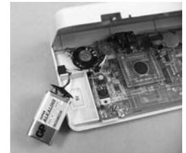
The battery life, (9 volt alkaline battery), is approximately two years if used only for backup.
