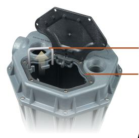
QuickTree<sup>®</sup> technology allows easy removal of float switch without disconnecting plumbing or pulling the pump.
