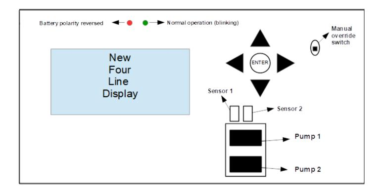
**Pump 1:** If system is a one pump system (X-Treme), make sure pump one is in the pump 1 slot.
