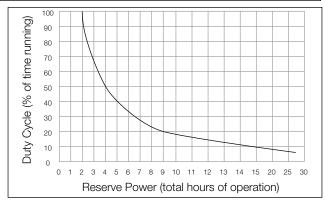
Performance curve results using a 3/4 HP pump with a 7.5 FLA and (2) Metropolitan Power Plus model 31P-36 batteries.
